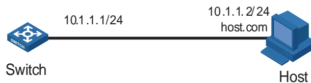
Figure 198 Network diagram for static DNS configuration
