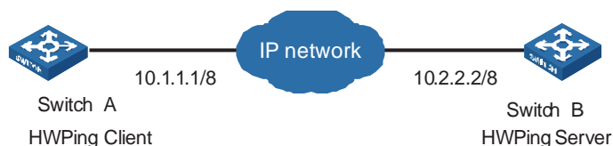
Figure 186 Network diagram for the Tcprivate test
