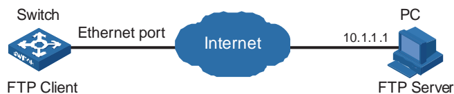
Figure 164 Remote loading using FTP Client
