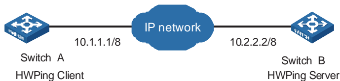
Figure 184 Network diagram for the Jitter test
