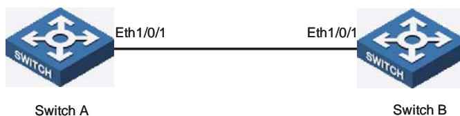
Figure 37 Network diagram for Ethernet port configuration
