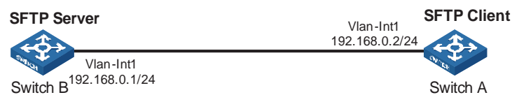
Figure 151 Network diagram for SFTP configuration
