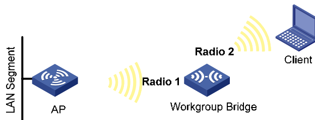
Figure 6-6 Network diagram for a workgroup bridge using two radio interfaces at the same time
