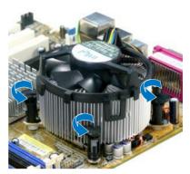
Pull up two fasteners at a time in a diagonal sequence to disengage the heatsink and fan assembly from the motherboard.
