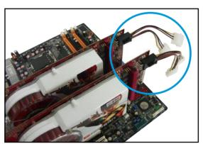
5. Connect one end of the external cable to the Master graphics card.
