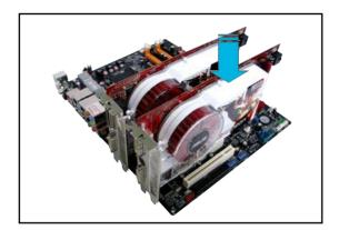
Connect an auxiliary power source from the power supply to the graphics cards.
