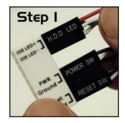
Install the ASUS Q-Connector to the system panel connector, making sure the orientation matches the labels on the motherboard.
