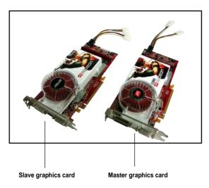
Insert the CrossFire<sup>™</sup> Edition (Master) graphics card into the PCI Express x16 <u>blue</u> slot. Make sure that the card is properly seated on the slot.
