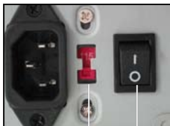
AC input voltage switch
