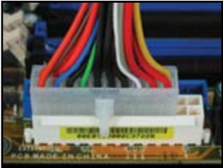
20-pin power connector (on the 24-pin female counterpart)
