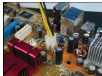
4-pin power connector (Konektor daya 4-pin)
