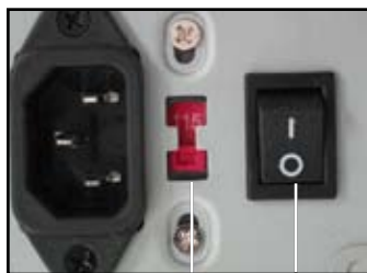
AC input voltage switch
