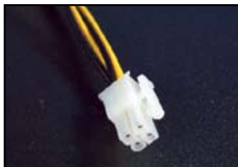
4-pin ATX connector
