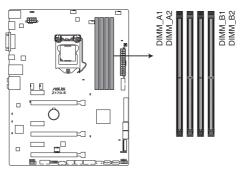
Z170-E 288-pin DDR4 DIMM socket
