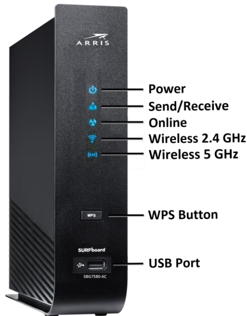
Figure 1: SBG7580-AC Front View
