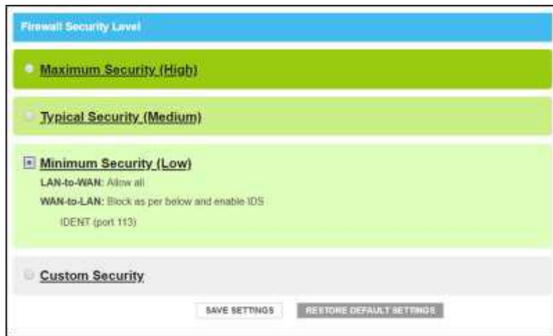
Figure 39: Firewall IPv4 low security level screen
