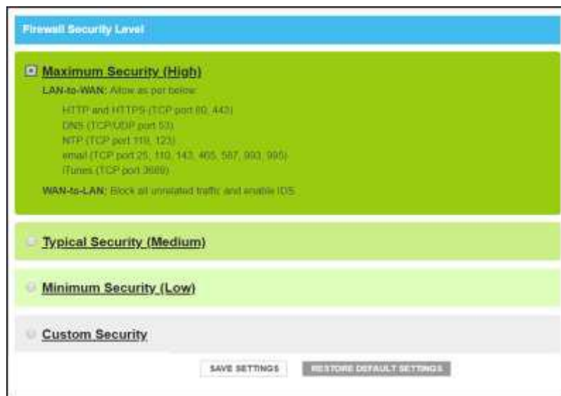
Figure 37: Firewall IPv4 high security level screen
