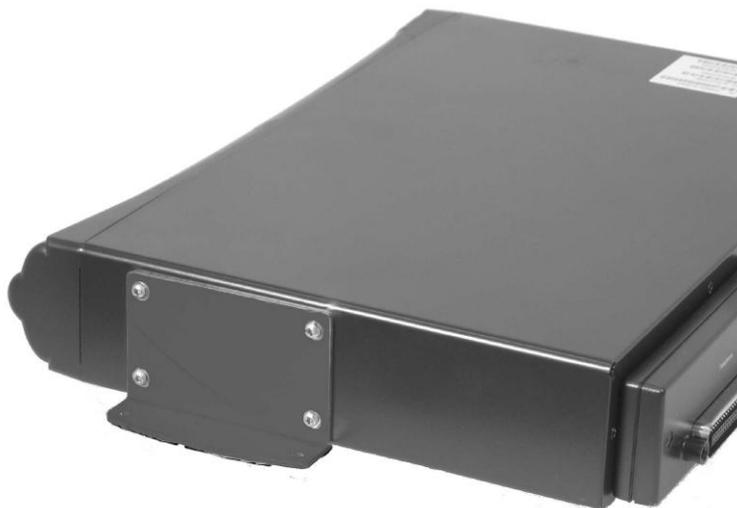
*Note:* Position the brackets so the bottom of the chassis will be against the mounting surface. This position leaves the serial number label exposed, and orients the front panel for best readability.
