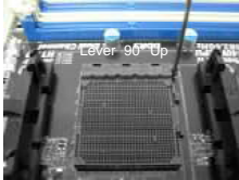
STEP 1: Lift Up The Socket Lever
