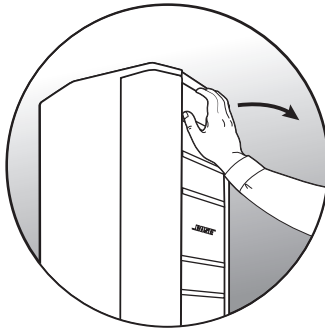
Pulling the array out
