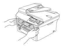
Pull out the drum unit and toner cartridge assembly.
