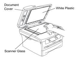
In the ADF unit, clean the white plastic bar and the scanner glass strip under it with isopropyl alcohol on a lint-free cloth.
