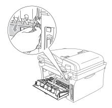
Pull the jammed paper out of the fuser unit. If the jammed paper cannot be pulled out easily, push down on the blue tab with one hand as you gently pull out the paper with the other hand.
