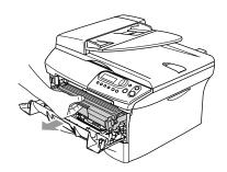
Clean the primary corona wire inside the drum unit by gently sliding the blue tab from right to left several times.
