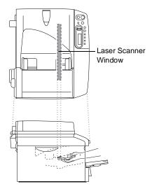
4 Put the drum unit and toner cartridge assembly back into the DCP.
