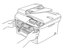
Pull out the drum unit and toner cartridge assembly.
