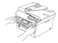
Pull out the drum unit and toner cartridge assembly. The jammed paper may be pulled out with the toner cartridge and drum unit assembly, or this may release the paper so you can pull it up and out of the paper tray opening.
