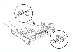
Fan the stack of paper well to avoid paper jams and mis-feeds.
