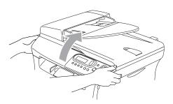
You can still use the DCP while the scanner cover is up. To close the scanner cover, push it down with both hands.
