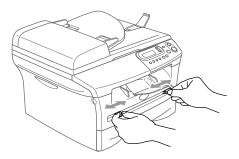
Using both hands put one sheet of paper in the manual feed slot until you feel the front edge of the paper touch the paper feed roller. Let go of the paper when you feel the DCP feed the paper in a short distance.
