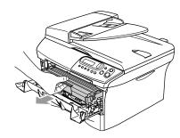
Hold down the lock lever on the left and pull the toner cartridge out of the drum unit
