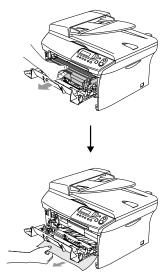
5 If you can not remove the drum unit and toner cartridge assembly easily, do not use extra force. Instead, lift the scanner cover and use both hands to carefully pull the jammed paper up and out of the output tray opening.
