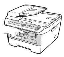
Slowly take out the drum unit and toner cartridge assembly. The jammed paper will be pulled out with the toner cartridge and drum unit assembly.
