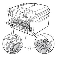
9 Pull the jammed paper out of the fuser unit.
