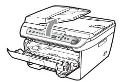
Use both hands to carefully pull the jammed paper up and out of the output tray opening.
