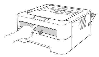
7 Using both hands, slide the manual feed paper guides to the width of the paper that you are going to use.
