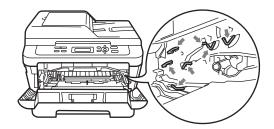
4 Put the print sample in front of the drum unit, and find the exact position of the poor print.
