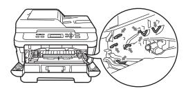
3 Push down the green lock lever and take the toner cartridge out of the drum unit.
