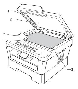
3 (For DCP-7065DN) In the ADF unit, clean the white bar (1) and the glass strip (2) underneath it with a soft lint-free cloth moistened with water.
