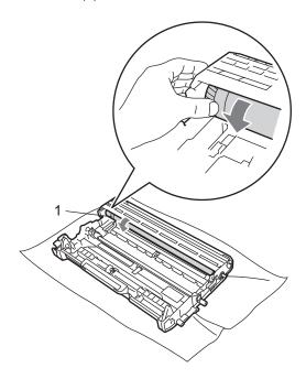
6 When you have found the mark on the drum that matches the print sample, wipe the surface of the OPC drum with a *dry* cotton swab until the dust or glue on the surface comes off.
