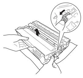
Put the toner cartridge back into the drum unit until you hear it lock into place. If you put the cartridge in correctly, the green lock lever on the drum unit will lift automatically.
