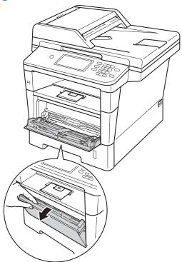
3 Pull out the MP tray support (1) and unfold the flap (2).
