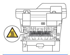
Using both hands, gently pull the jammed paper out of the back of the machine.
