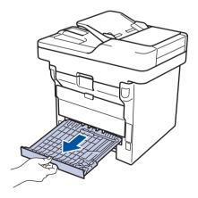
Pull the jammed paper out of the machine or out of the 2-sided tray.
