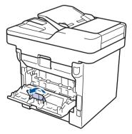
On the front of the machine, open the MP tray and lower it gently.
