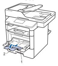
Slide the MP tray paper guides to fit the width of the paper that you are using. If the paper guide on the right side has a lever, press it and slide the paper guide.
