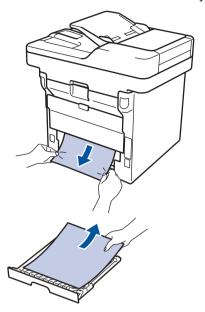
Remove paper that may have jammed under the machine due to static electricity.
