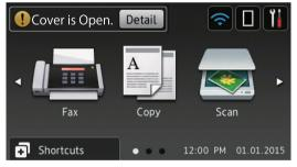
The warning icon appears when there is an error or maintenance message; press Detail to view it, and then press to return to Ready Mode.
