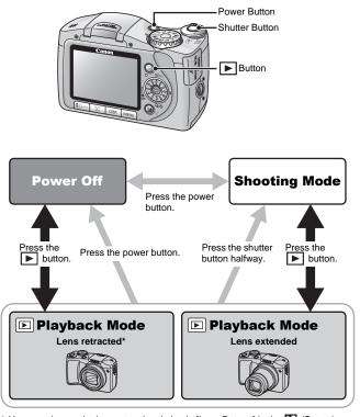
\* You can change the lens retraction timing in [Lens Retract] in the (Set up) menu (p. 49).
