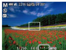
Aperture Value Shutter Speed Standard Exposure Level Exposure Level Indicator Exposure Level Mark
