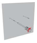
Align the holes on the back of the Device with the screws on the wall. Hang the Device on the screws.
