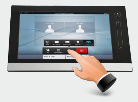
The EX90 can be configured via the touch screen controller or via its web interface. For full access to all configurable parameters the web interface must be used—the touch screen controller provides access to a limited set of parameters only.
