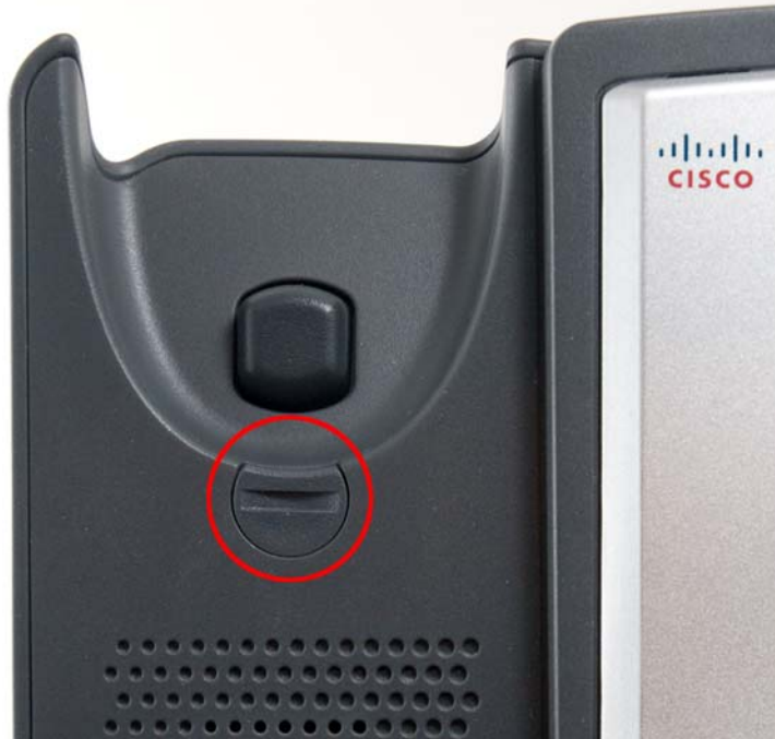
Figure 5 Handset Retention Tab (Default Position)
