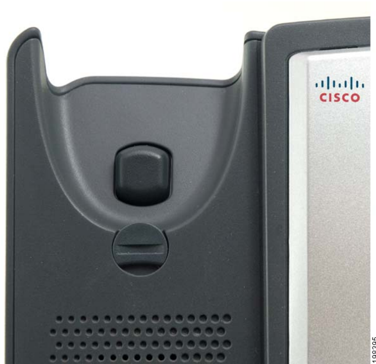
Figure 6 Handset Retention Tab (Reversed)
