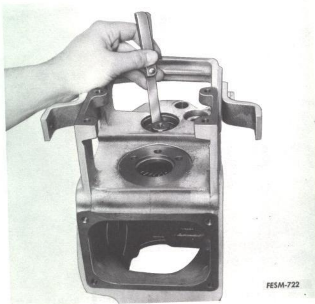
Illustr. 2-72. Measuring snap ring groove gap.
