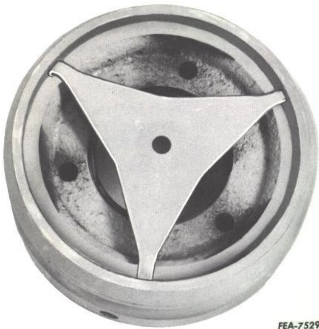
Illust. 2-84. Pressure spring located on pulley.
