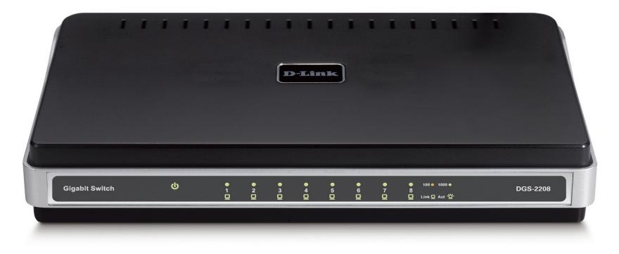
The LED indicators of the Switch include Power, 100/1000Mbps, and Link/Act. The following shows the LED indicators for the Switch along with an explanation of each indicator.
