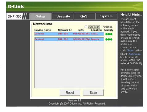
Red text on the **Device Name**, **Network ID**, **MAC** & **Location** columns mean that the powerline network is encrypted with the default Network ID (DHP-300). Follow the steps below to encrypt the network with a non-default Network ID:
