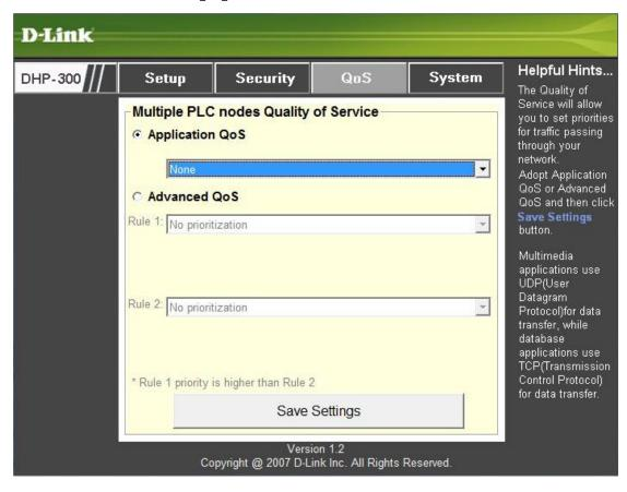
The Quality of Service (QoS) screen will allow you to set priorities for traffic passing through your network. By default all types of traffic are assigned the same priority. Multimedia applications use UDP (User Datagram Protocol) for data transfer, while database applications use TCP (Transmission Control Protocol) for data transfer.
