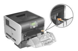
The envelope feeder tilts downward at a slight angle when it is installed properly.
