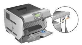
6. Insert the hook on the bottom of the cardboard cover retainer into the slot on the printer. You will need to lower the top front cover to do this.
