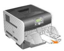
If the jammed envelope has entered the printer and cannot be pulled out, remove the envelope feeder.
