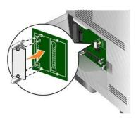
4. Push the Font ROM firmly into place, and release the locking clips.
