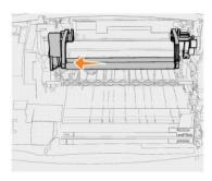
9. Pull the charge roll to the right and out of the printer.
