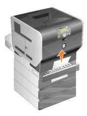
Open any optional trays beginning at the top, and remove any jammed media.
