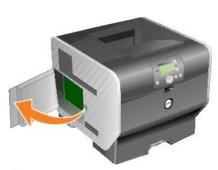
NOTICE: Printer memory memory cards are easily damaged by static electricity. Touch something metal such as the printer frame before you touch a memory card.
