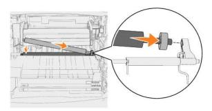
10. Lower the transfer roller gently until the left metal tab fits into the slot. You may have to push it down for a secure fit.
