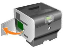
NOTICE: Option cards are easily damaged by static electricity. Touch something metal such as the printer frame before you touch an option card.
