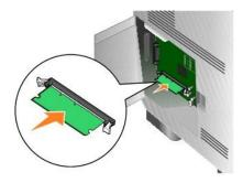
6. Make sure each latch fits over the notch on the end of the card.
