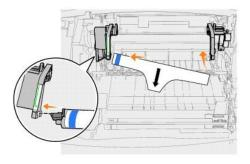
11. Lift the right side of the charge roll and insert it into its hole.
