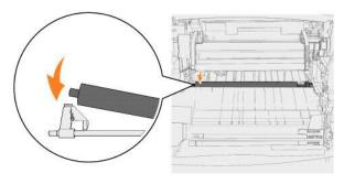
11. Reinstall the print cartridge into the printer.
