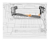
10. Align the blue tab on the left side of the charge roll with its hole in the arm marked with the corresponding blue arrow, and insert it. Pull the charge roll to the left.
