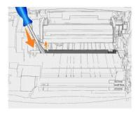
7. Lift the transfer roll and pull it straight out of the printer. Set it aside.
