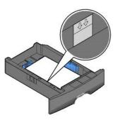
6. Squeeze the side guide tab, and slide the guide toward the inside of the tray until it lightly rests against the edge of the media.
