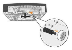
5. Repeat  $\underline{\text{step 3}}$  and  $\underline{\text{step 4}}$  on the other side to remove the other pick roller.
