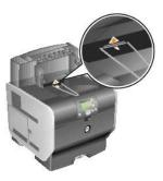
5. Slide the lower tabs on the tray into the lower slots on the output expander.
