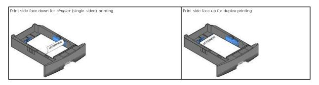
NOTE: Do not fill paper above the load line. Overfilling the tray may cause jams.
