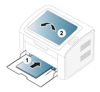
4 Squeeze the paper width guide and slide it to the edge of the paper stack without causing it to bend.
