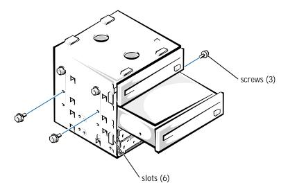
9 With the slots on the drive cage extending slightly beyond the front of the computer, lower the drive cage and slide it toward the back of the computer until the cage locks into place.
