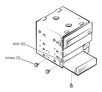
To install a new drive in the upper 3.5-inch bay, first remove the 1/4-inch screw and drive bracket from the drive cage. Attach the new drive to the bracket with two drive screws on the right side. Then slide the drive into the drive bay and secure it to the drive cage with one 1/4-inch screw on each side.
