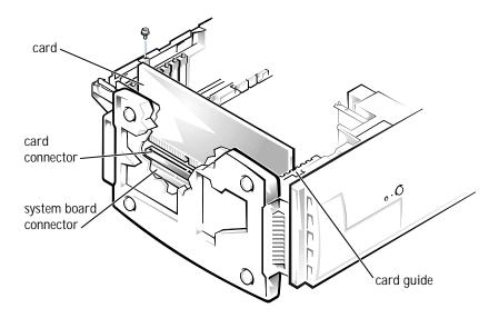
Make sure that the card is fully seated and that its bracket is within the card slot.
