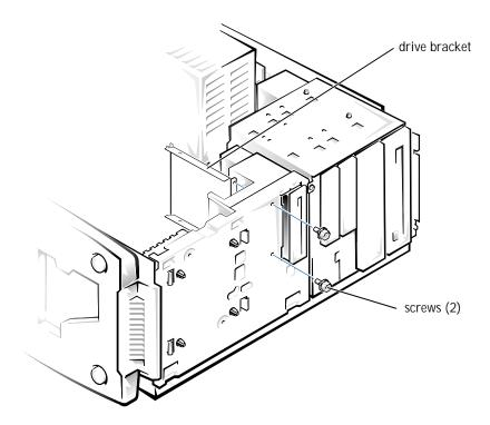
6 Orient the new drive with its circuit board facing the inside of the bracket. Align the bracket tabs with the two tab holes in the side of the drive, and rotate the drive into the bracket. Then secure the screw.
