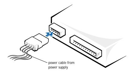
NOTICE: When you attach the extra connector to the new drive in the following step, match the colored strip on the cable with pin 1 on the drive. 11 Remove the tape from the wide cable connector and reattach the connector to the original drive. Locate the extra connector on the cable and attach it to the new drive.
