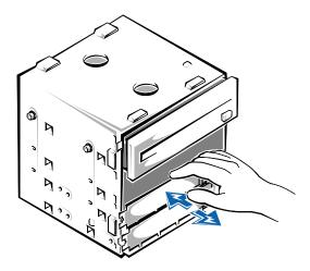
To install a new drive in the lower 3.5-inch bay, slide the drive into the bay and secure it with three screws.
