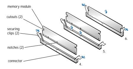
To remove a memory module, press out the securing clip at each end of the memory connector until the memory module disengages from the connector.
