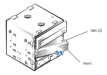
Slide the new drive into the bay, and secure the drive with the three screws.
