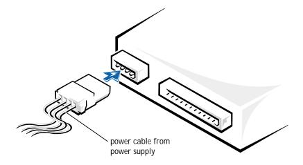
NOTICE: When you attach the extra connector to the new drive in the following step, match the colored strip on the cable with pin 1 on the drive. 12 Remove the tape from the wide cable connector and reattach the connector to the original drive. Locate the extra connector on the cable and attach it to the new drive.
