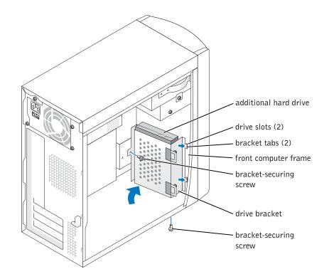
**12** Reinstall the existing hard drive into the computer in front of the additional drive.
