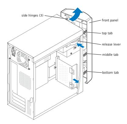
c Rotate the front panel to separate it from the side hinges.
