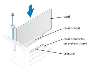
Ensure that the card is fully seated and that its bracket is within the card slot.
