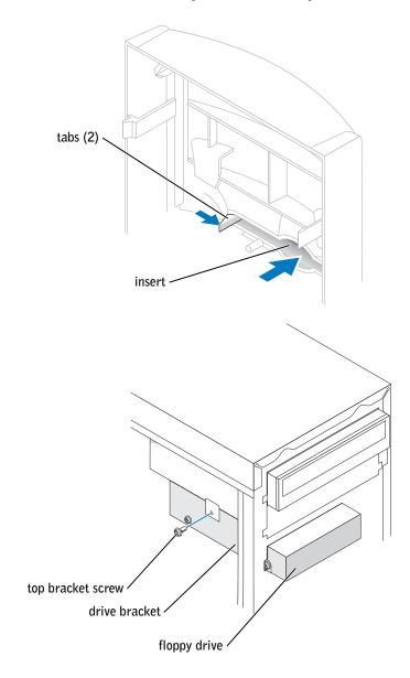
7 Press in the two insert tabs, and then push out the front-panel insert.
