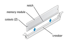
9 Align the notch on the bottom of the module with the crossbar in the connector.
