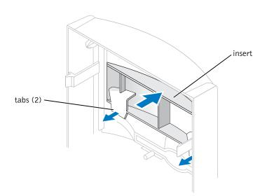
7 Pull the two front-panel tabs towards you, and then push out the front-panel insert.
