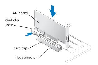
2 Release the card lever, ensuring that the tab fits into the notch on the front end of the card.
