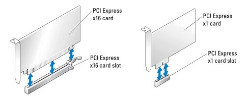
If you are installing or replacing a PCI Express card, follow the procedures in the next section. If you are removing but not replacing a PCI Express card, see "Removing a PCI Express Card" on page 68.
