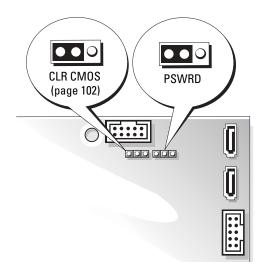
**2** Locate the 3-pin password jumper (PSWD) on the system board (see page 56), and attach the jumper plug to pins 2 and 3 to clear the password.
