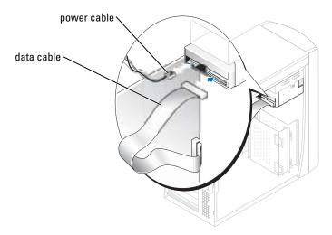
NOTICE: Match the colored strip on the cable with pin 1 on the drive (pin 1 is marked as "1").
