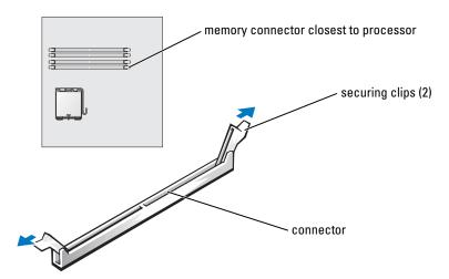
3 Press out the securing clip at each end of the memory module connector.
