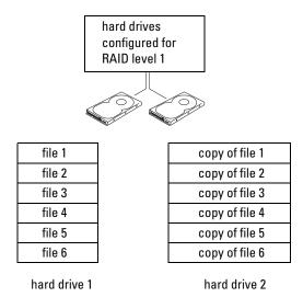
If a drive failure occurs, subsequent read and write operations are directed to the surviving drive. A replacement drive can then be rebuilt using the data from the surviving drive.
