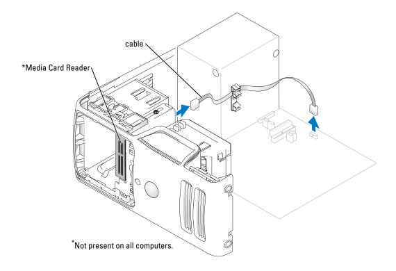
**5** Disconnect the FlexBay USB cable on the back of the Media Card Reader from the Media Card Reader connector on the system board (see "System Board Components" on page 67) and route the cable through the cable routing clip.
