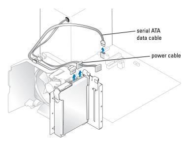
Press in on the blue tabs on each side of the drive and slide the drive up and out of the computer.
