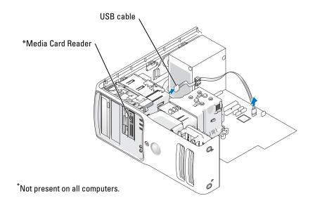
5 Disconnect the USB cable on the back of the Media Card Reader to the front panel USB connector on the system board (see page 63) and route the cable through the clip on the shroud.
