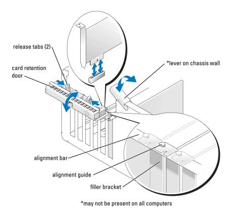
If present on your computer, rotate the lever on the chassis wall upward.
