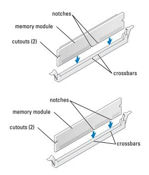
**NOTICE:** To avoid damage to the memory module, press the module straight down into the connector while you apply equal force to each end of the module.
