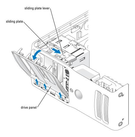
2 Grasping the lever on the sliding plate, pull the sliding plate to the right and hold in place.**NOTE:** The sliding plate secures and releases the drive panel and helps to secure the drives.
