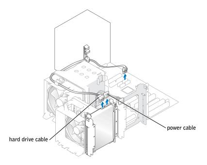
2 Press in on the tabs on each side of the drive and slide the drive up and out.
