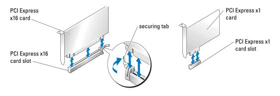
NOTICE: Ensure that you release the securing tab to unseat the card. If the card is not removed correctly, the system board may be damaged.
