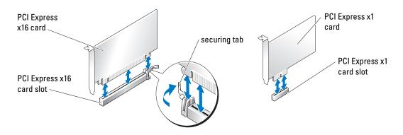
• NOTICE: Ensure that you release the securing tab to unseat the card. If the card is not removed correctly, the system board may be damaged.
