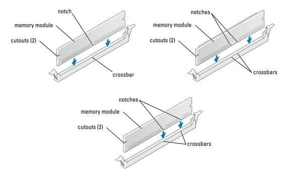
**5** Align the notch on the bottom of the module with the crossbar in the connector.
