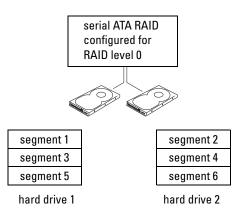
Another advantage of a RAID level 0 configuration is that it utilizes the full capacities of the drives. For example, if you have two 120-GB drives installed, you have 240 GB on which to store data.
