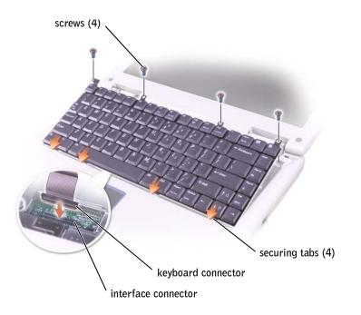
**9** Insert the four securing tabs on the keyboard into their respective slots in the palm rest, and lower the keyboard into the bottom case.
