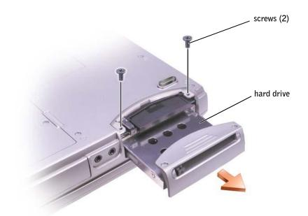
**NOTICE:** When the hard drive is not in the computer, store it in protective antistatic packaging. See "Protecting Against Electrostatic Discharge" on page 17.
