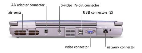
**AIR VENTS** — The computer uses an internal fan to create airflow through the vents, which prevents the computer from overheating.
