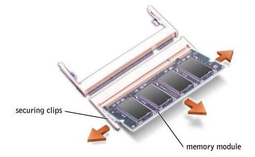
**NOTE:** If the memory module is not installed properly, the computer may not boot properly. No error message indicates this failure.
