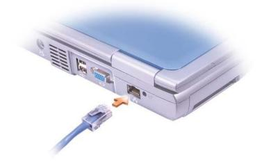
**NOTE:** Do not use a network cable with a telephone wall jack.
