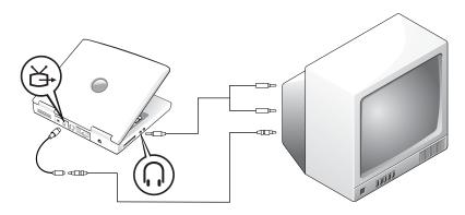
To connect the computer to a television that has a composite video input only, use a composite TV-out adapter cable:
