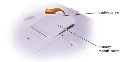
**3** Remove the screw labeled "O" next to the memory module cover.
