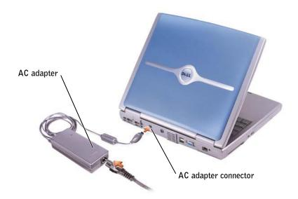
**NOTE:** The fan runs constantly, and fan speed may vary depending on usage. Fan noise is normal and does not indicate a problem with the fan or the computer. The AC adapter converts AC power to the DC power required by the computer. You can connect the AC adapter with your computer turned either on or off.
