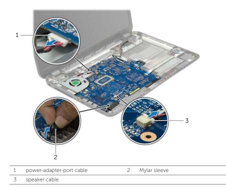
Removing the System Board | **39**
