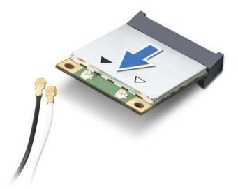
CAUTION: When the Mini-Card is not in the computer, store it in protective antistatic packaging. For more information, see "Protecting Against Electrostatic Discharge" in the safety information that shipped with your computer.
