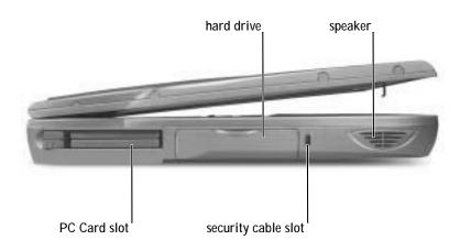
PC CARD SLOT — Has two connectors that support various types of PC Cards, including modems and network adapters. For more information, see the Tell Me How help file. To access the help file, see page 56.
