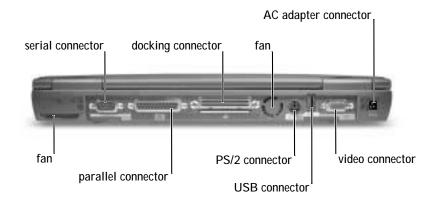
**FAN** — The computer uses an internal fan to create airflow through the vents, which prevents the computer from overheating.
