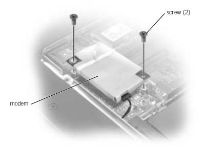
**2** Connect the modem cable to the modem.
