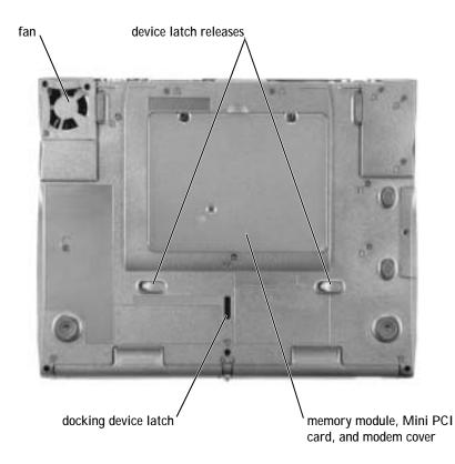
**FAN** — The computer uses an internal fan to create airflow through the vents, which prevents the computer from overheating.
