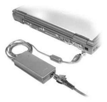
The AC adapter converts AC power to the DC power required by the computer. You can connect the AC adapter with your computer turned either on or off.
