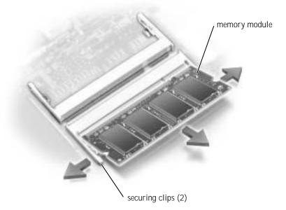
**NOTICE:** If you need to install memory modules in two connectors, install a memory module in the connector labeled "JDIM (DIMMA)" before you install a module in the connector labeled "JDIM2 (DIMMB)."
