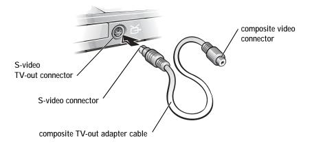
**3** Plug one end of the composite video cable into the composite video connector on the composite TV-out adapter cable.
