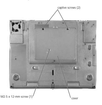
7 Remove the screw(s) from the cover, and lift up the cover.
