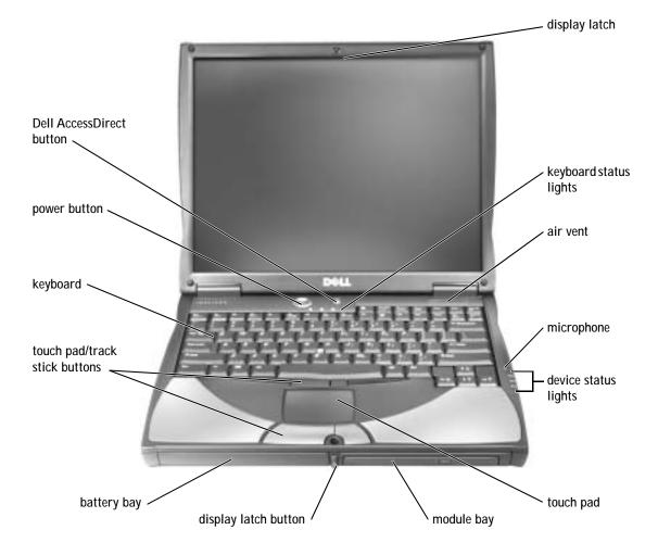
**DISPLAY LATCH** — Keeps the display closed.
