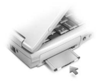
The computer recognizes most PC Cards and automatically loads the appropriate device driver. If the configuration program tells you to load the manufacturer's drivers, use the floppy disk or CD that came with the PC Card
