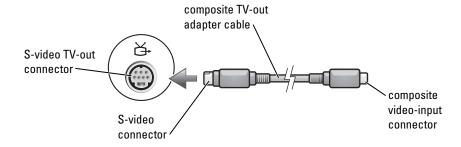
**3** Plug one end of the composite video cable in to the composite video-input connector on the composite TV-out adapter cable.
