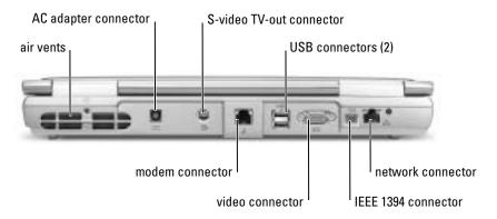
**AIR VENTS** — The computer uses an internal fan to create airflow through the vents, which prevents the computer from overheating.
