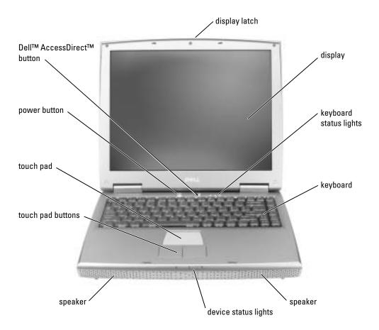
**DISPLAY LATCH** — Keeps the display closed.
