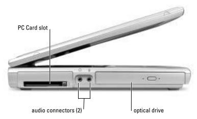
**PC CARD SLOT** — Supports one PC Card, such as a modem or network adapter. For more information, see "Using PC Cards" in the *Dell Inspiron Help* file. To access the help file, see page 10.
