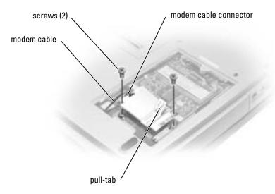
**5** Connect the modem cable to the modem.
