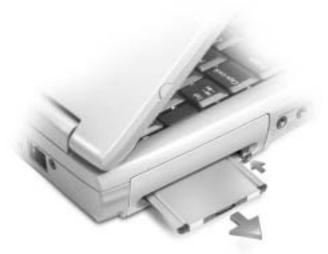
**3** Save a blank to use when no PC Card is installed in a slot. Blanks protect unused slots from dust and other particles.
