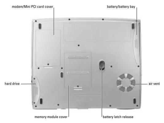
MODEM/MINI PCI CARD COVER — Covers the compartment that contains the modem and Mini PCI card. See page 87.
