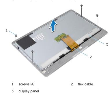
**16** Remove the screws that secure the display-panel brackets to the display panel.
