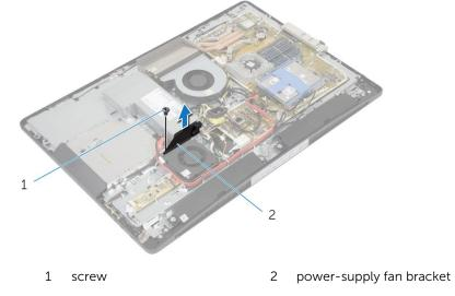
3 Disconnect the power-supply fan cable from the power-supply unit.
