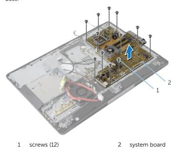
**3** Gently lift the system board at an angle and remove the side I/O bracket off the system board.
