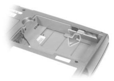
3 Pull the reserve battery out of its compartment, and disconnect the reserve battery cable from the connector.
