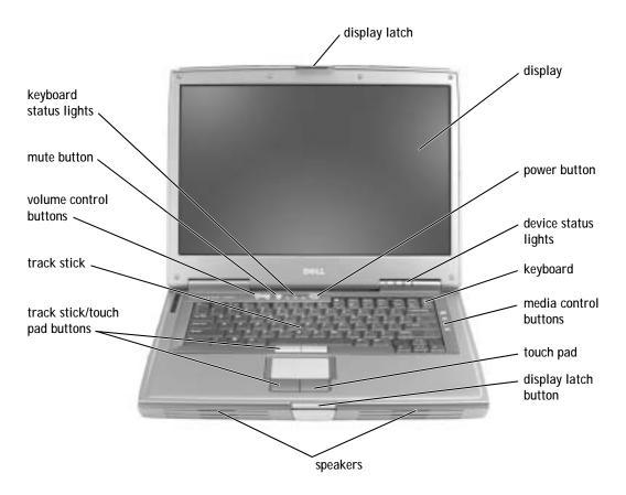
**DISPLAY LATCH** — Keeps the display closed.
