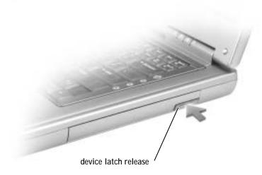
2 Pull the device out of the module bay.
