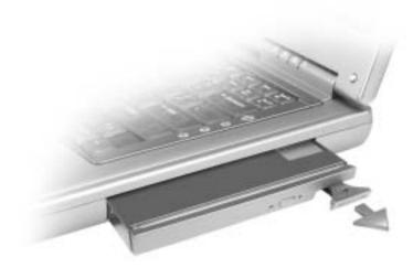
3 Insert the new device into the bay, and push the device until you feel a click.
