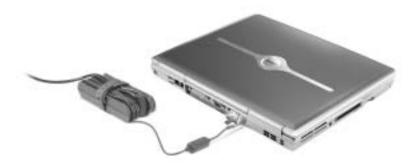
The AC adapter converts AC power to the DC power required by the computer. You can connect the AC adapter with your computer turned either on or off.
