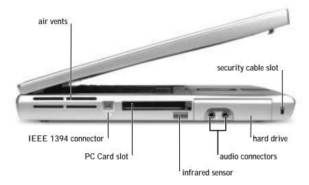
AIR VENTS — The computer uses an internal fan to create airflow through the vents, which prevents the computer from overheating.
