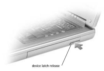
4 Pull the device out of the module bay.
