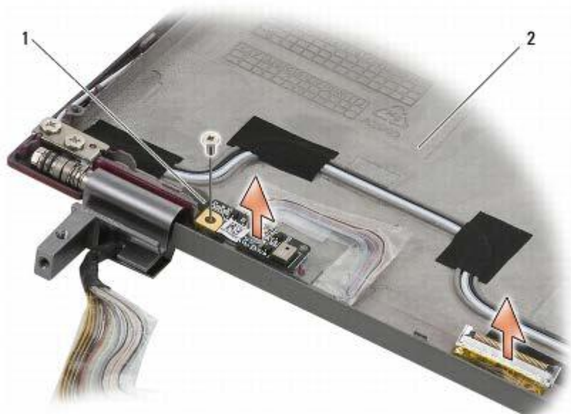
1 LCD cable board 2 display back cover
