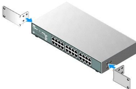
Figure 1-7. Brackets for Rack Installation
