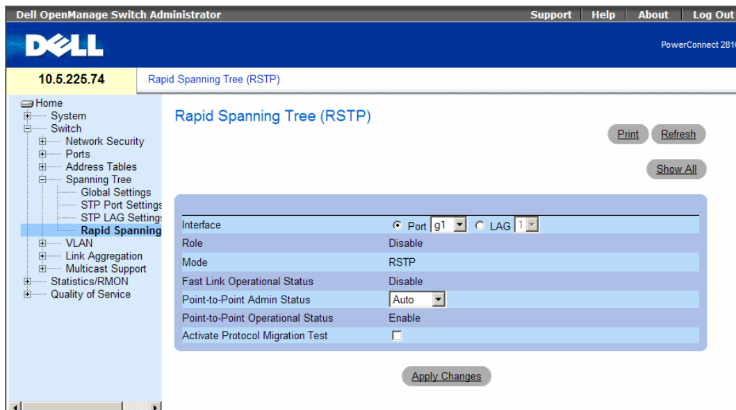
Figure 7-19. Rapid Spanning Tree (RSTP)
