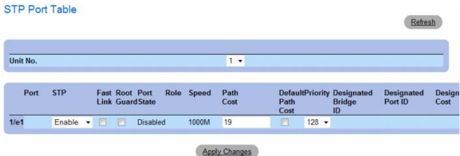
Figure 7-37. STP Port Table
