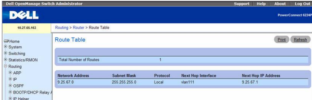
Figure 9-35. Router Route Table
