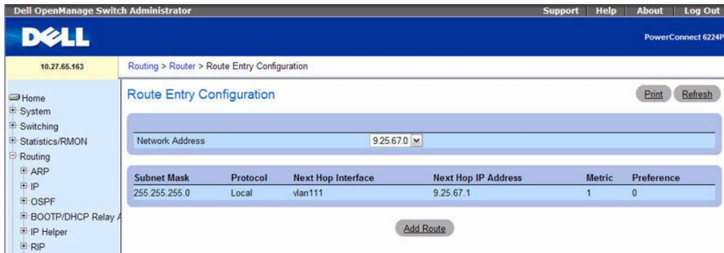
Figure 9-37. Router Route Entry Configuration
