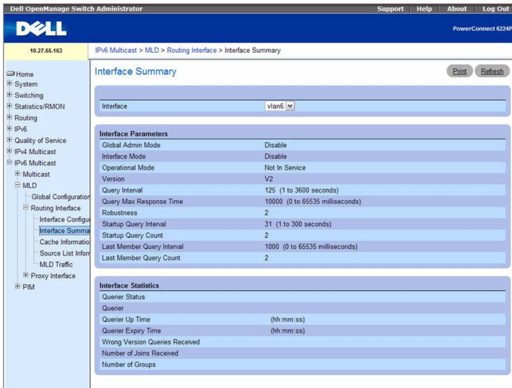
Figure 12-25. MLD Routing Interface Summary
