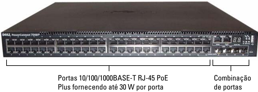
Figura 1-5. PowerConnect 7048P com 48 portas 10/100/1000BASE-T PoE Plus
