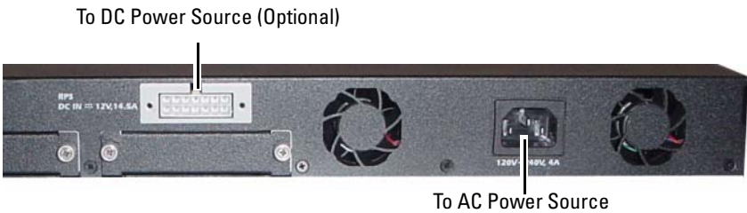
Figure 1-15. AC and DC Power Connection to Switch
