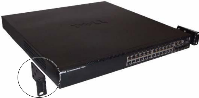
Figure 1-11. Attaching the Brackets
