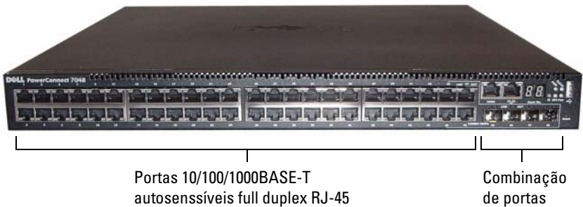
Figura 1-4. PowerConnect 7048 com 48 portas 10/100/1000BASE-T
