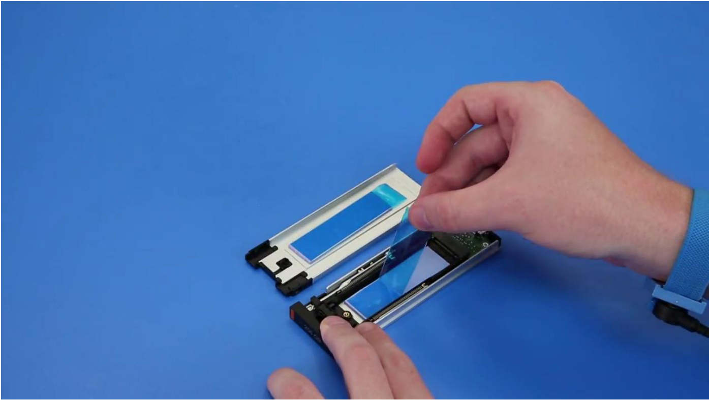
c. Peel off the adhesive tape from the SSD carrier cover.
