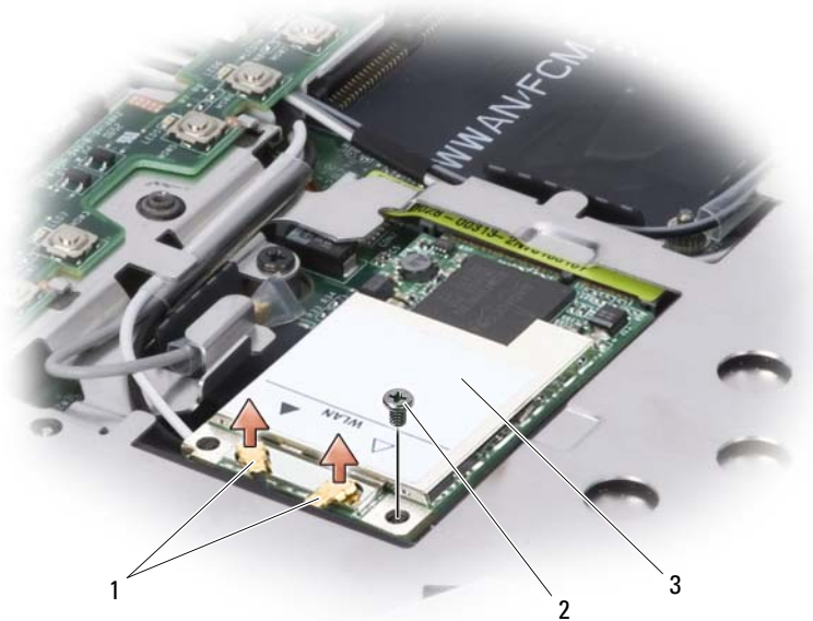
1 antenna cable connectors 2 screw 3 WLAN card
