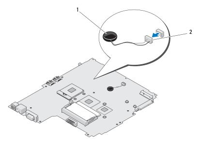
1 coin-cell battery 2 coin-cell battery cable connector
