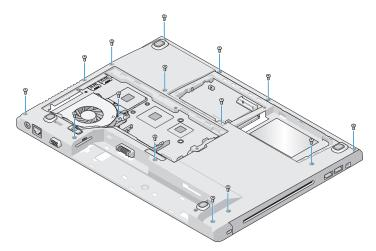
Turn the computer over and remove the three M2.5 x 5-mm screws that secure the top of the palm rest.
